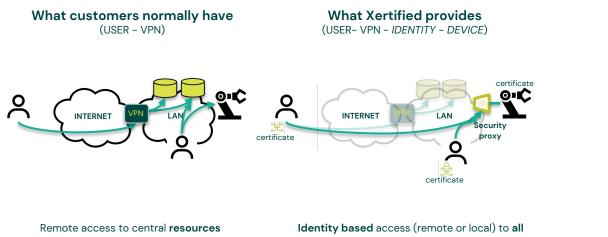
Remote access to central **resource** through a classical Virtual Private Network (VPN) solution or local access with low security Identity based access (remote or local) to all connected physical devices. Encryption endto-end from any connected physical device to the end-user laptop/tablet/phone
